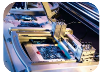
Six Sigma repeatability at class-leading accuracy of +/- 12.5 microns
